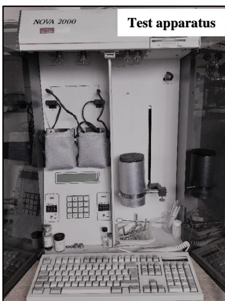
**Figure 5-43 (a): Surface area apparatus**
