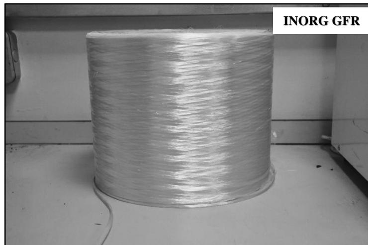
**Figure 5-22: Glass fibre doff**
