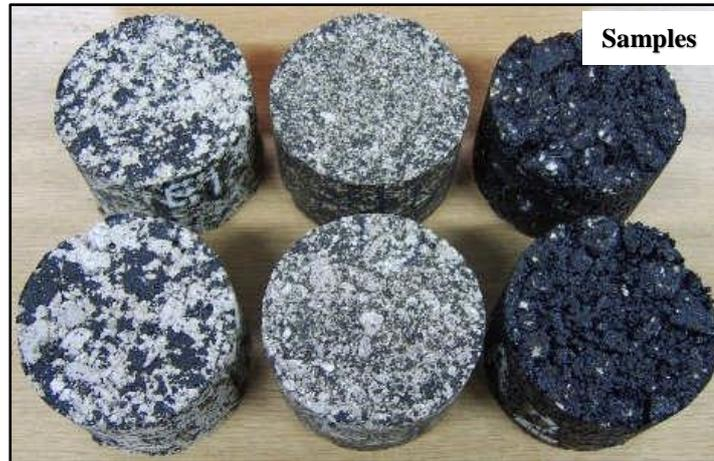
**Figure 3-13: Difference between cold mix (left: grey) and hot mix (right: black)**
