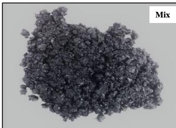
**Figure 5-28: Microasphalt mix prepared in the laboratory**
