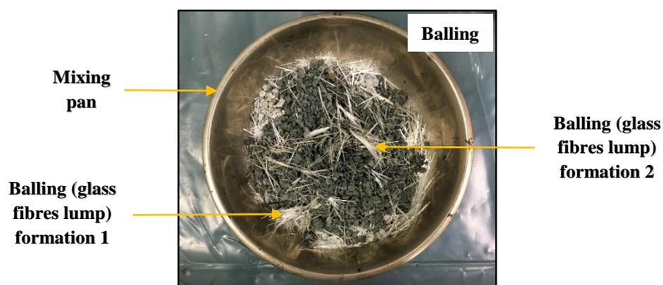
**Figure 6-1: Balling phenomenon in microasphalt**
