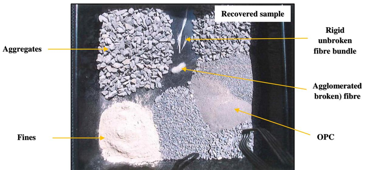
**Figure 7-10: Two forms of glass fibre and aggregates recovered from a site sample**
