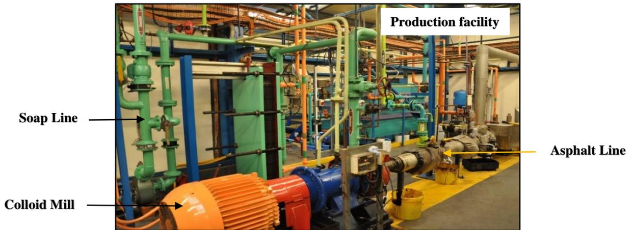
**Figure 5-17: Bitumen emulsion production facility**
