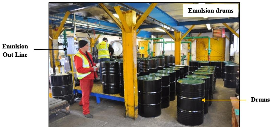
**Figure 5-20: Drums filled with bitumen emulsion**
