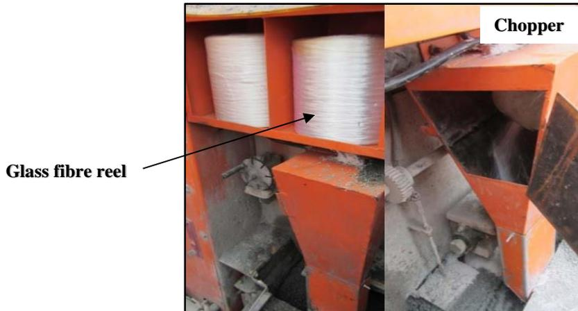
**Figure 7-6: Two reels of glass fibre with a chopper (open cover)**
