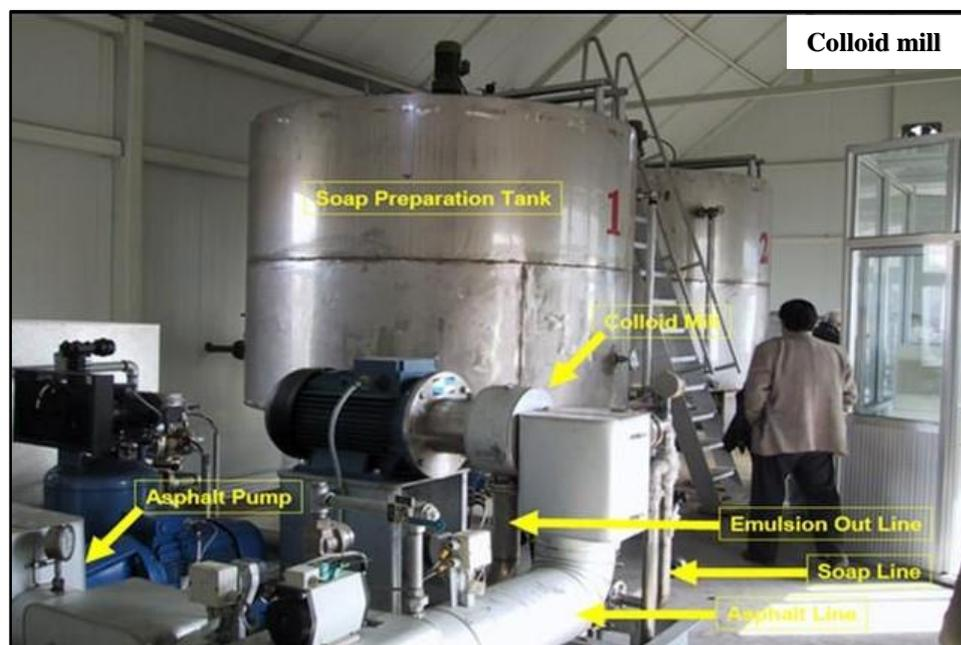
**Figure 3-5: Bitumen emulsion - colloid mill**
