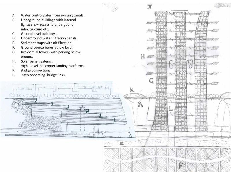
Example of Ground Source Energy Station integration in large -scale Eco-City such as Zhenzhou,
