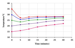
Fig. 3 Effect of Initial Temperature on ECR1 Performance (i=  $1mA/cm^2$  and E= 0.15 mS/cm).
