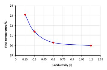
Fig. 4 Effect of water conductivity on water temperature (i= $1 \text{mA/cm}^2$ , T =20 min)
