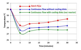
Fig. 2 Comparison among the studied reactors in term of temperature behavior (i= 1mA/cm<sup>2</sup> and E= 0.15 mS/cm)
