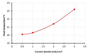
Fig. 5 Effect of Current Density on Water Temperature (conductivity = 0.6 mS/cm, T =20 min)
