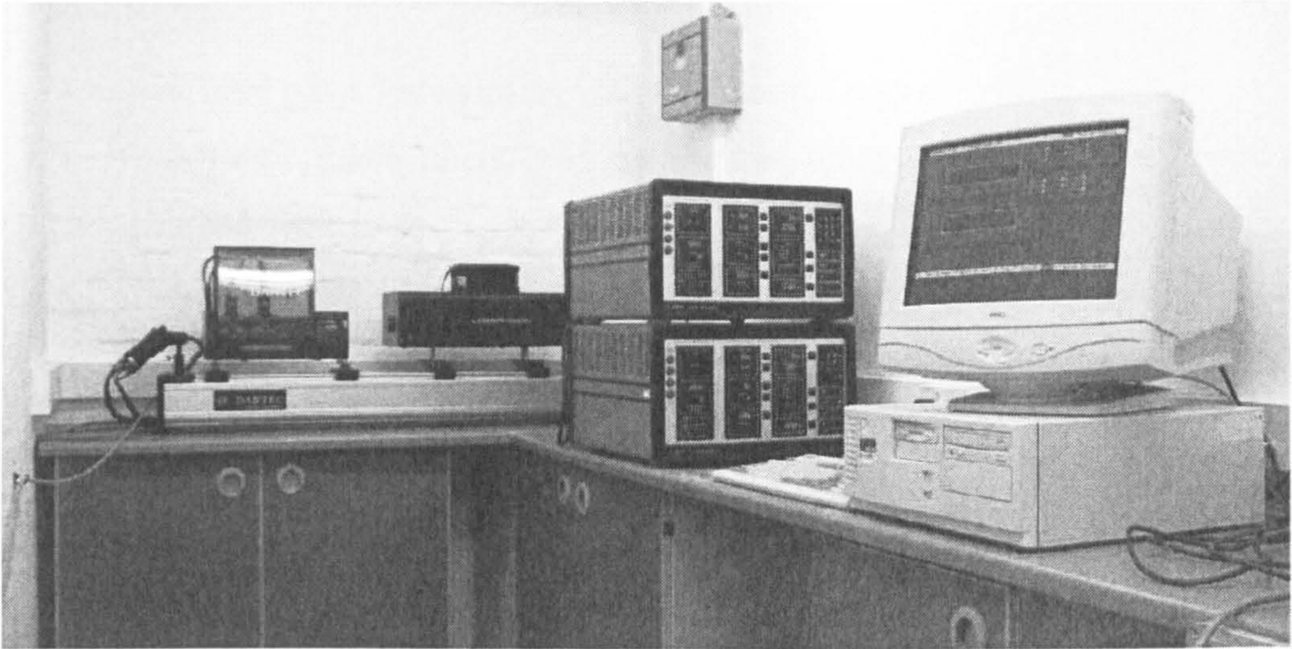
Figure 3-4 Laser Doppler Anemometry measuring system setup
