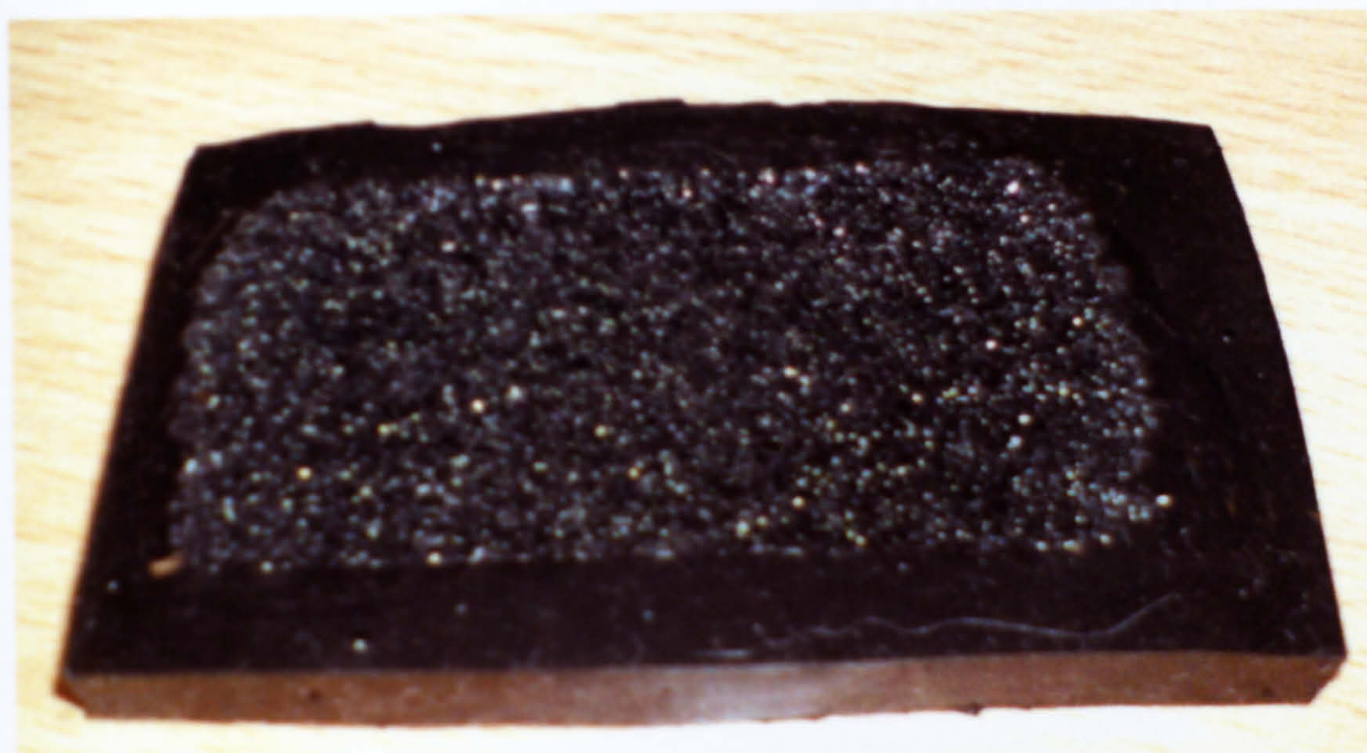
Example of Microset impression of the surface the Altos wheel.
