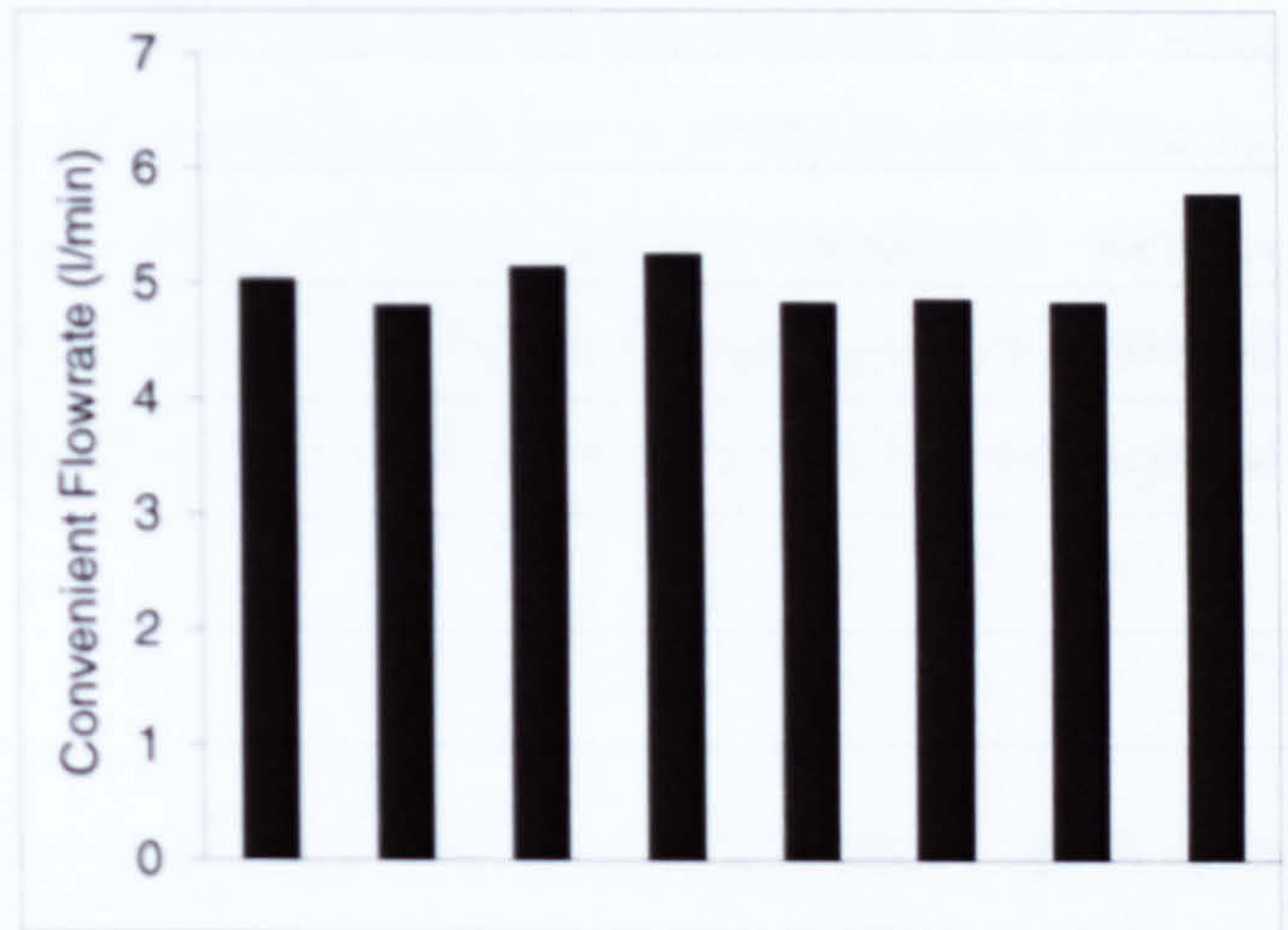
Figure 77, Convenient flowrate approximations from all topography tests with the Flexovit wheel when v_s=30 m/s.
