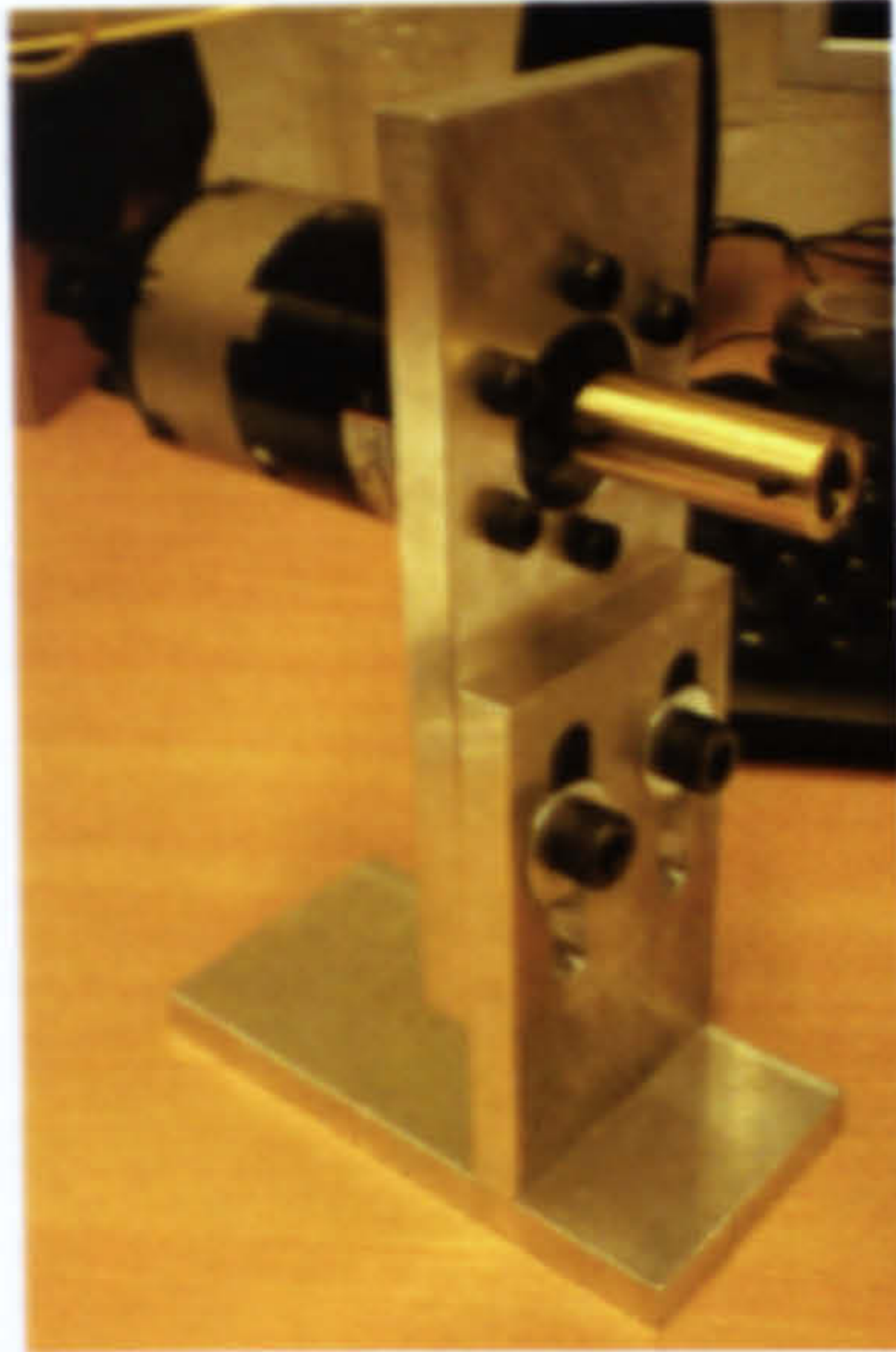
SMC Rotary actuator mounted to the stand and with the coupling attached.
