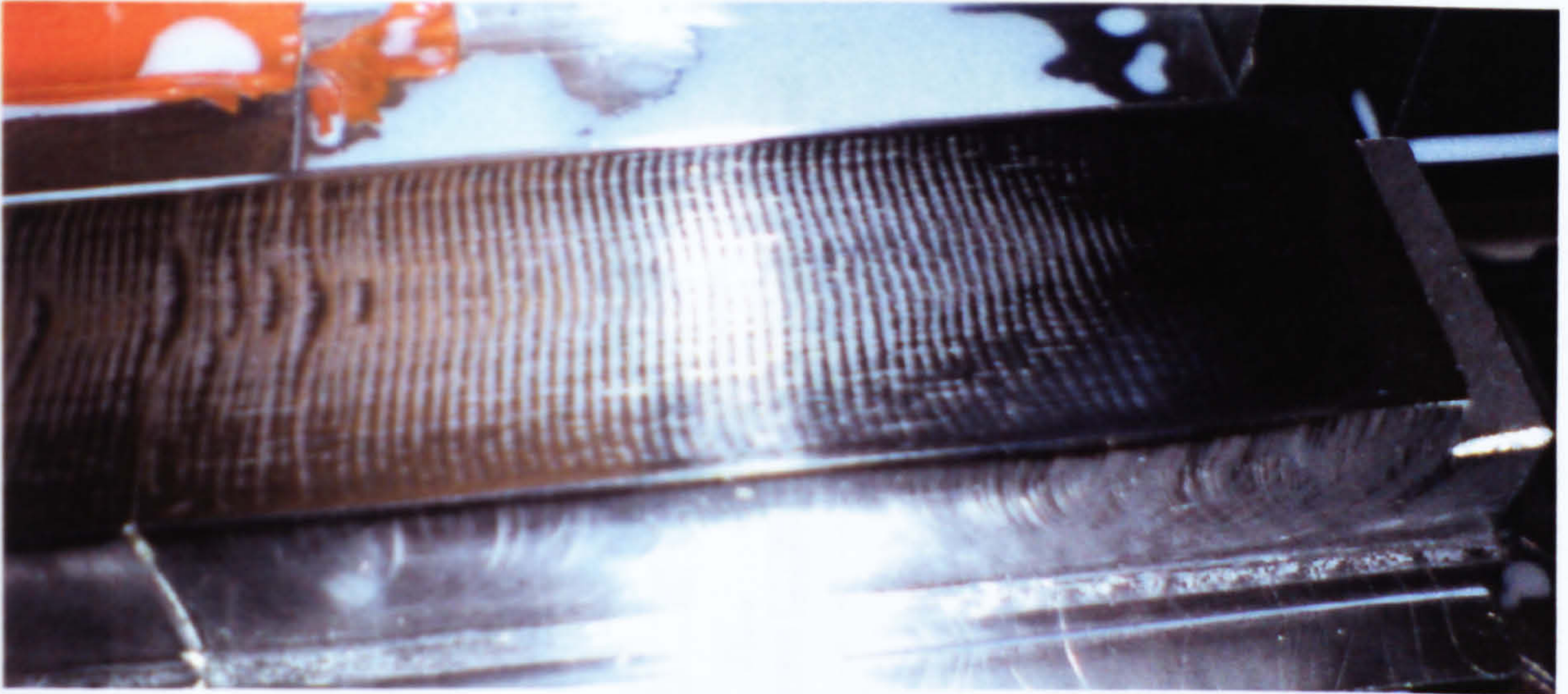
Burn of O1 workpiece during Taguchi tests.
