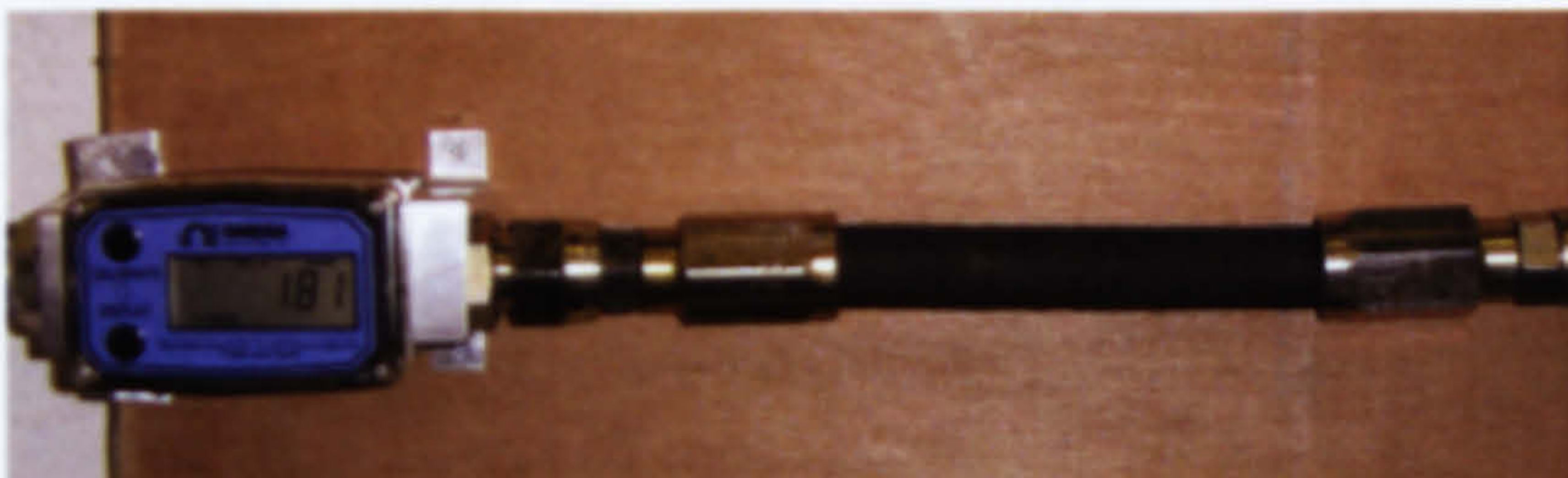
Figure 17, Flowmeter showing straight lead inlet section.
