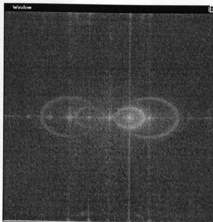
*Figure 88. Symmetrical reflectance produced by mis-calibration of the system.*
