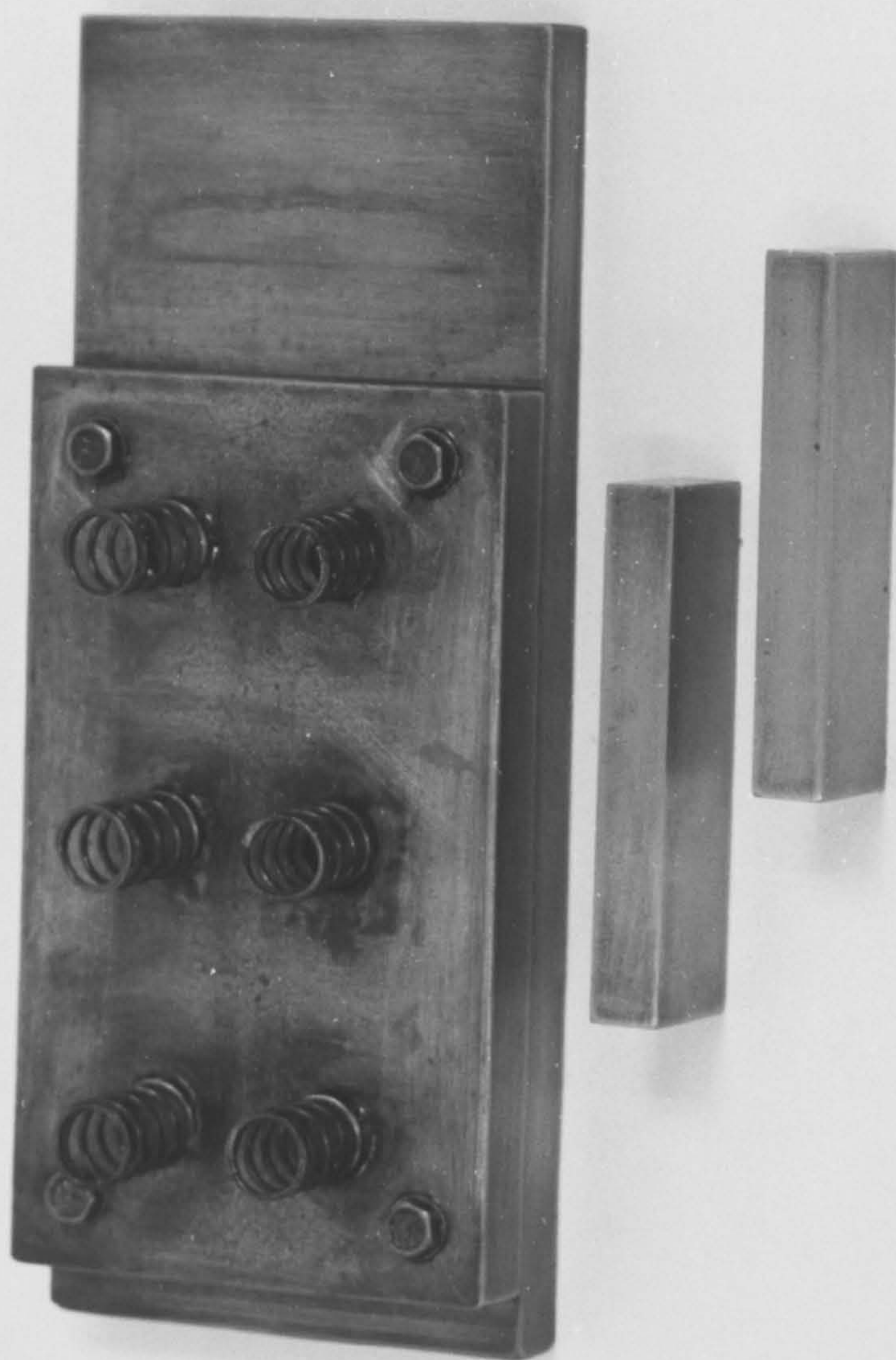
Figure 7.5 - Grading bar mould and compression platen.
