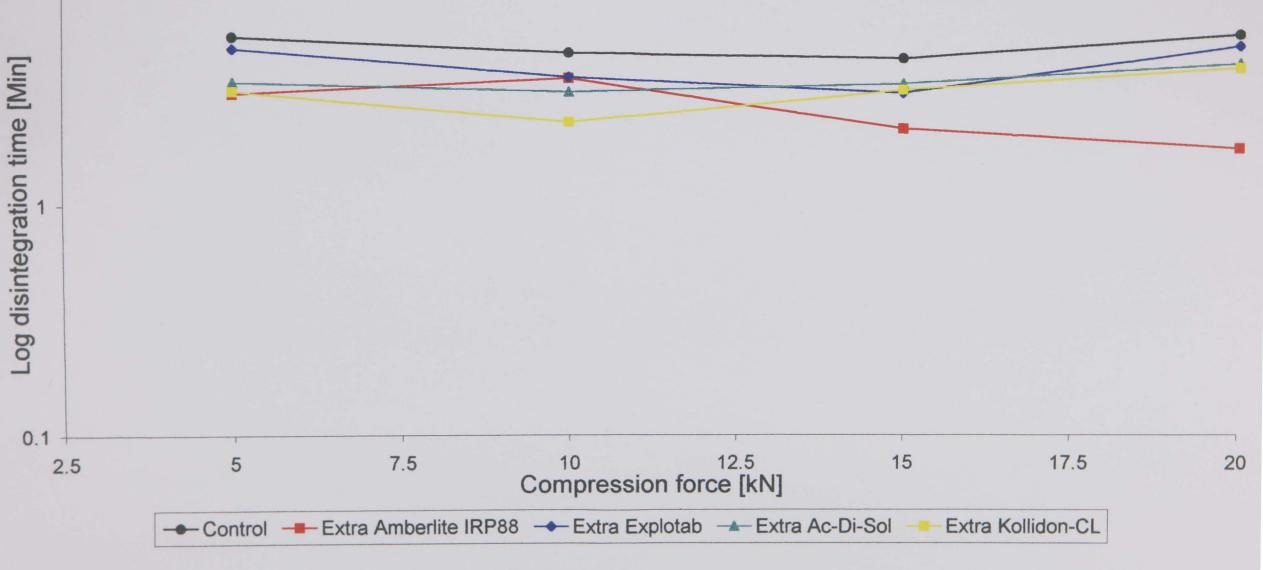
Figure 4.3: Effect of extragranular disintegrant type / compression force on the disintegration of tablets containing intragranular Ac-Di-Sol through a screen aperture size of 710 $\mu$ m.
