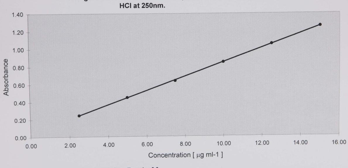
Figure 2.7: Calibration curve of paracetamol In methanolic HCI at 250nm.
