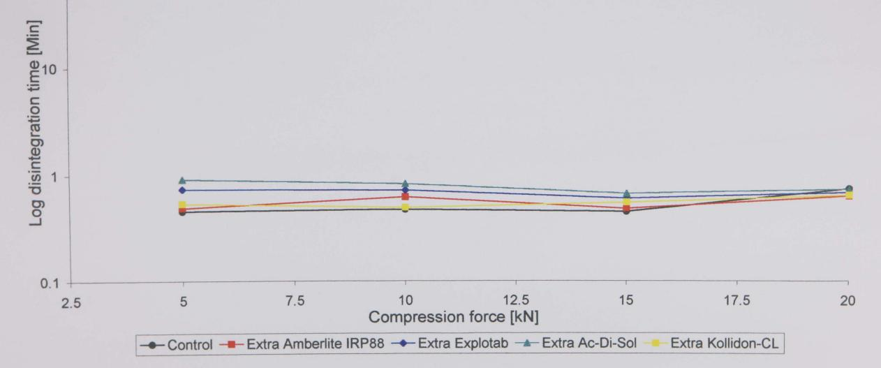
Figure 4.4: Effect of extragranular disintegrant type / compression force on the disintegration of tablets containing intragranular Kollidon-CL through a screen aperture size of 710 $\mu$ m.
