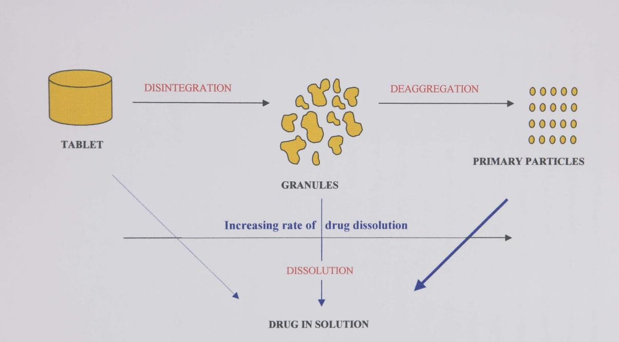
Figure 1.4: Disintegration, deaggregation and dissolution in the breakdown of solid oral dosage forms (after Wagner 1969, Wells, 1980).
