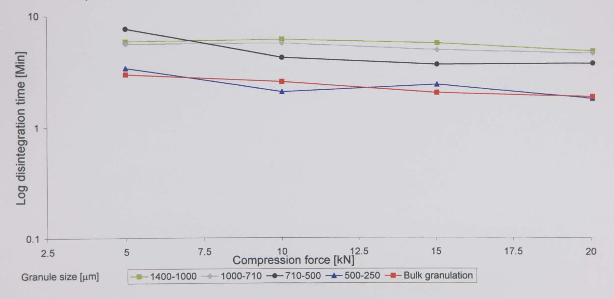
Figure 3.14: Effect of granule size / compression force on the disintegration of tablets containing 2% intragranular Amberlite IRP88 through a screen aperture size of  $1400\mu m$ .
