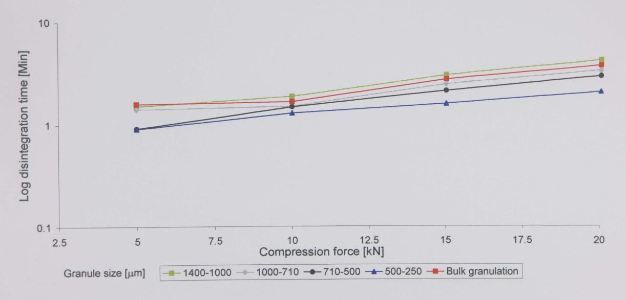
Figure 3.11: Effect of granule size / compression force on the disintegration of tablets containing 2% intragranular Explotab through a screen aperture size of 1180 $\mu$ m.
