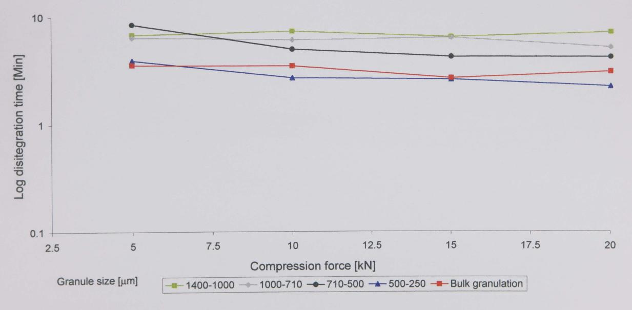
Figure 3.15: Effect of granule size / compression force on the disintegration of tablets containing 2% intragranular Amberlite IRP88 through a screen aperture size of  $1180\mu m$ .
