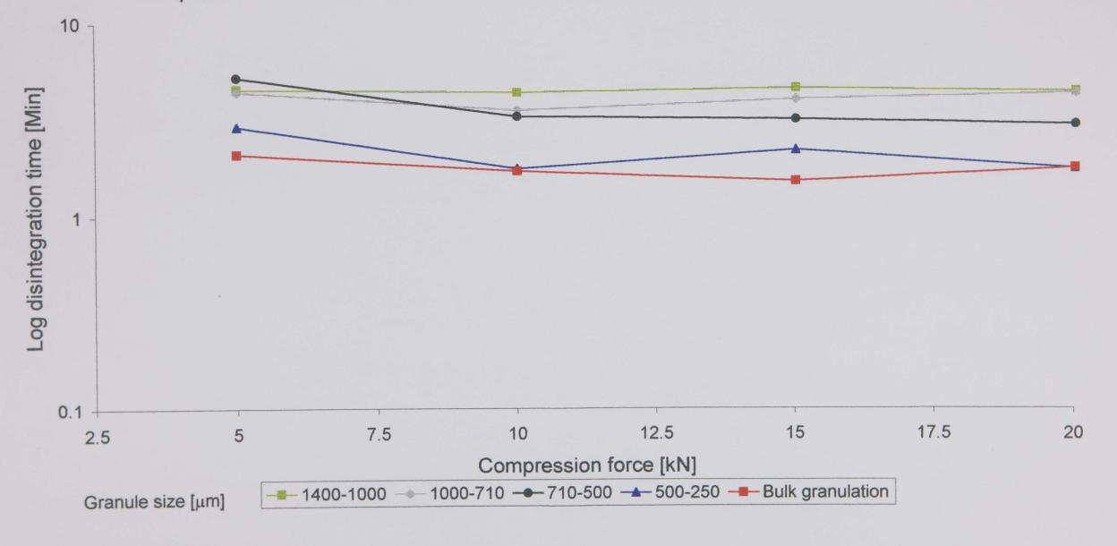
Figure 3.13: Effect of granule size / compression force on the disintegration of tablets containing 2% intragranular Amberlite IRP88 through a screen aperture size of  $1700\mu m$ .
