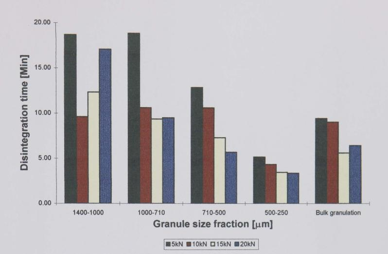
Figure 3.7: Effect of granule size / compression force on the disintegration of tablets containing 2% intragranular Amberlite IRP88 through 710µm.
