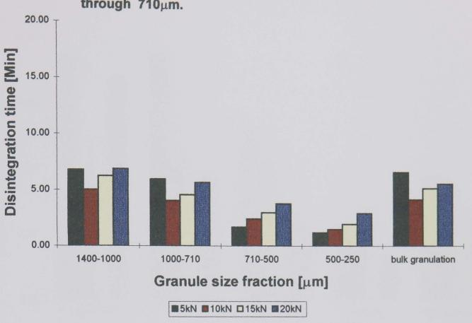
Figure 3.5: Effect of granule size / compression force on the disintegration of tablets containing 2% intragranular Explotab through 710 $\mu$ m.
