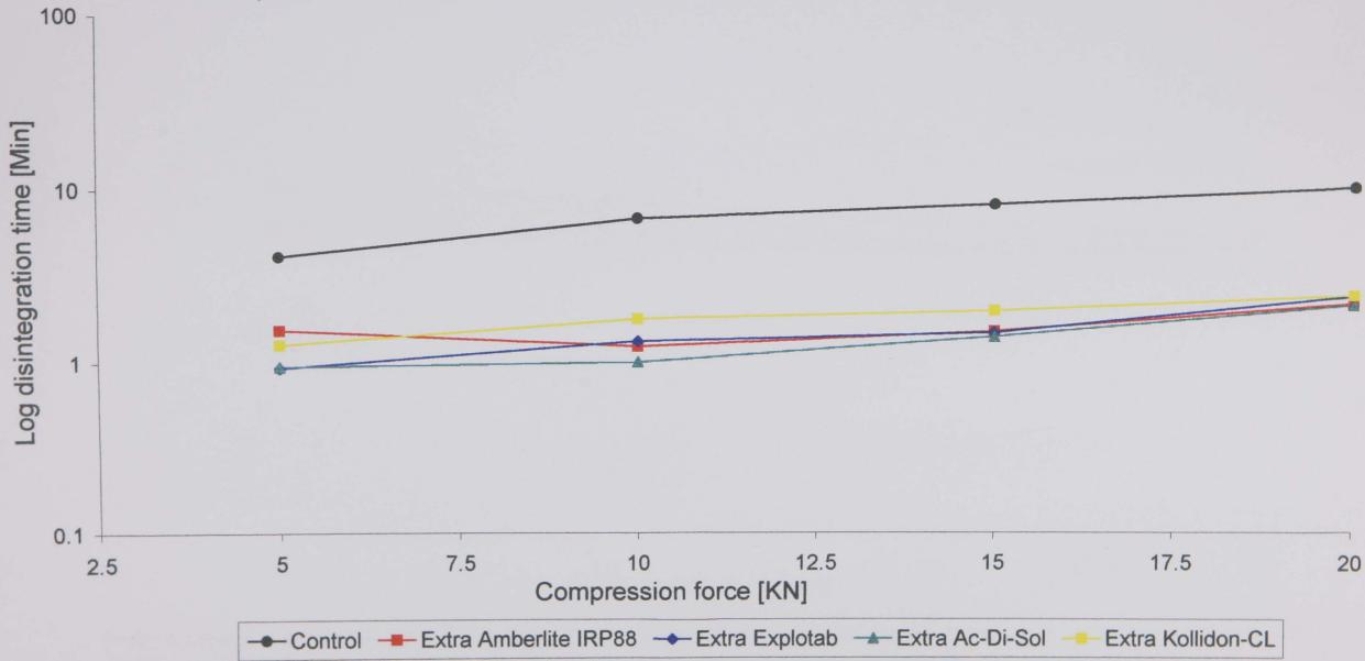
Figure 4.5: Effect of extragranular disintegrant type / compression force on the disintegration of tablets containing intragranular Amberlite IRP88 through a screen aperture size of  $710 \mu m$ .
