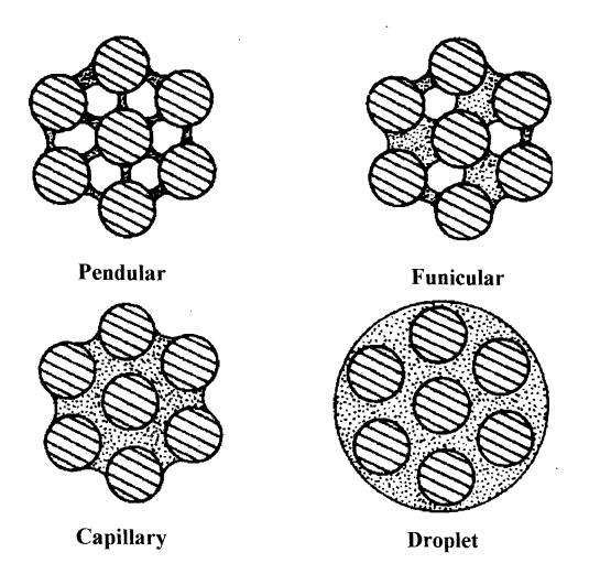
Figure 1.2: Binding mechanisms by liquid bridges.
