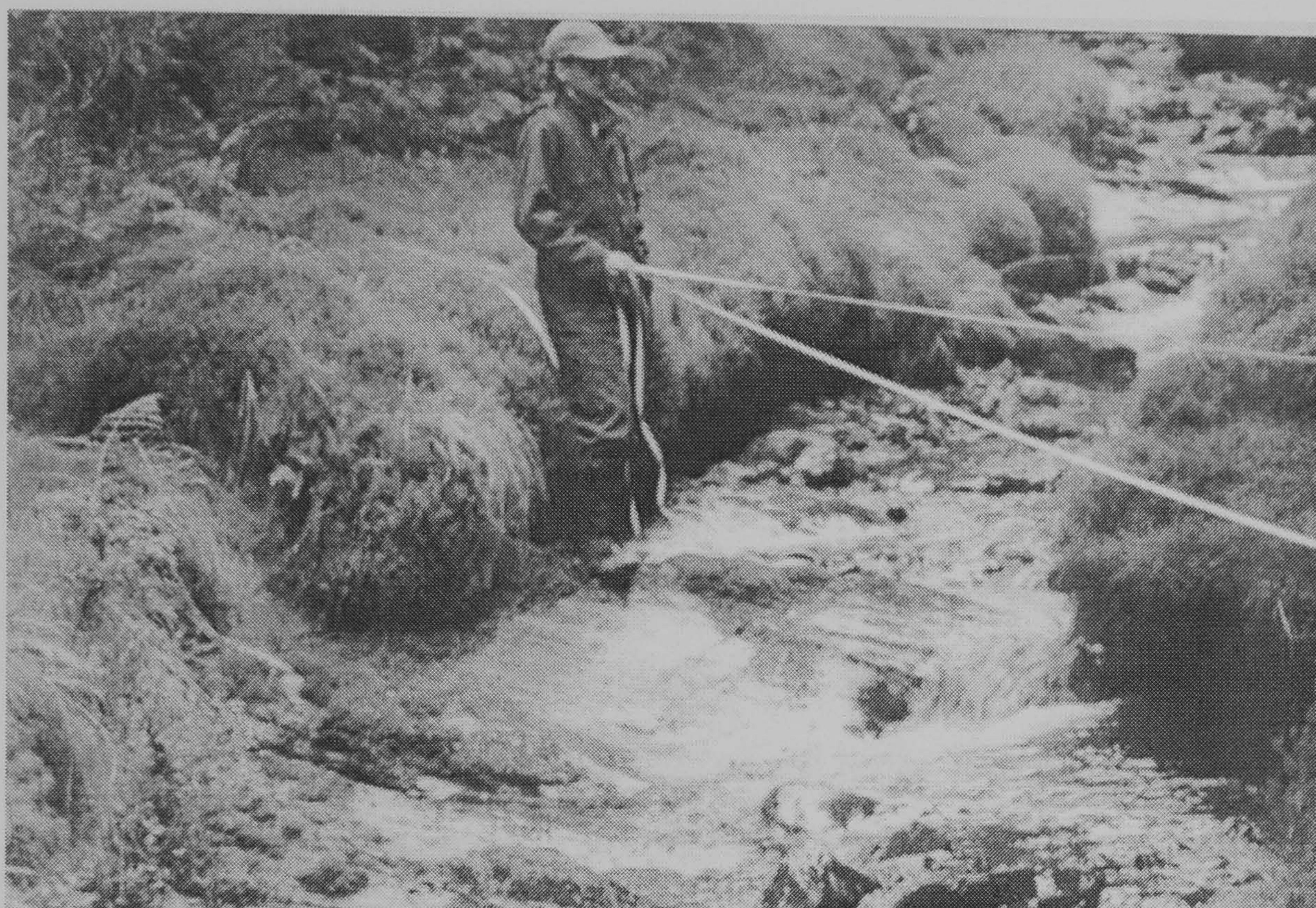
Plate 3.6. The two-tapes method. Tracer pebble location and mapping in the Nant Tanllwyth
