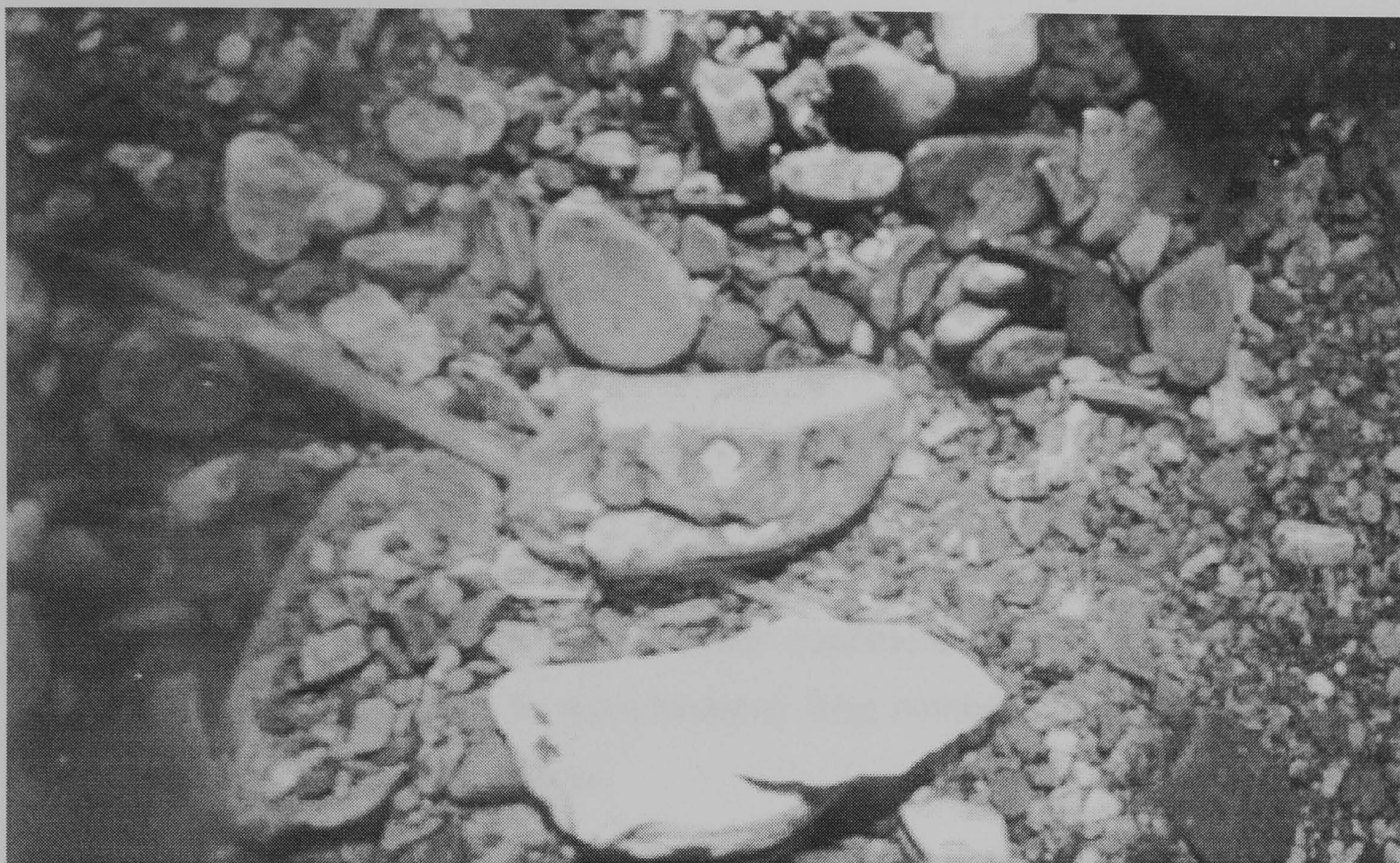
Plate 3.5. Labelled tracer clast in Nant Tanllwyth (above) with temporary marker pebble (below)
