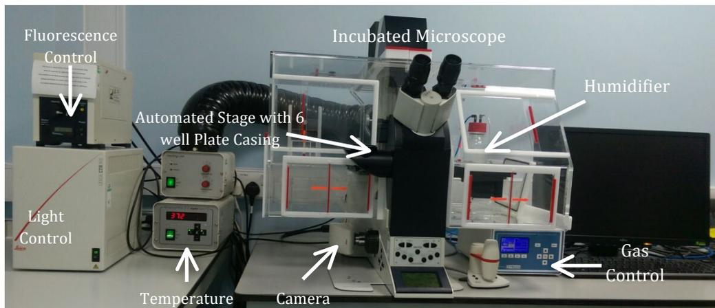
**Figure 3.13.** Annotated image of live imaging hardware used to perform live imaging experiments and fluorescence microscopy. Images are visualized via Leica Application Suite linked to the microscope.
