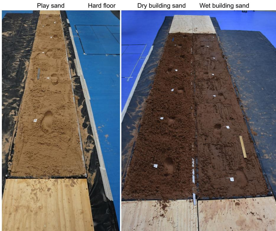
**Fig. 1. Example of the setup of the wooden walkways and substrates.** The four different substrates include play sand (far left), hard lab floor (centre left), dry building sand (centre right) and wet building sand (far right).
