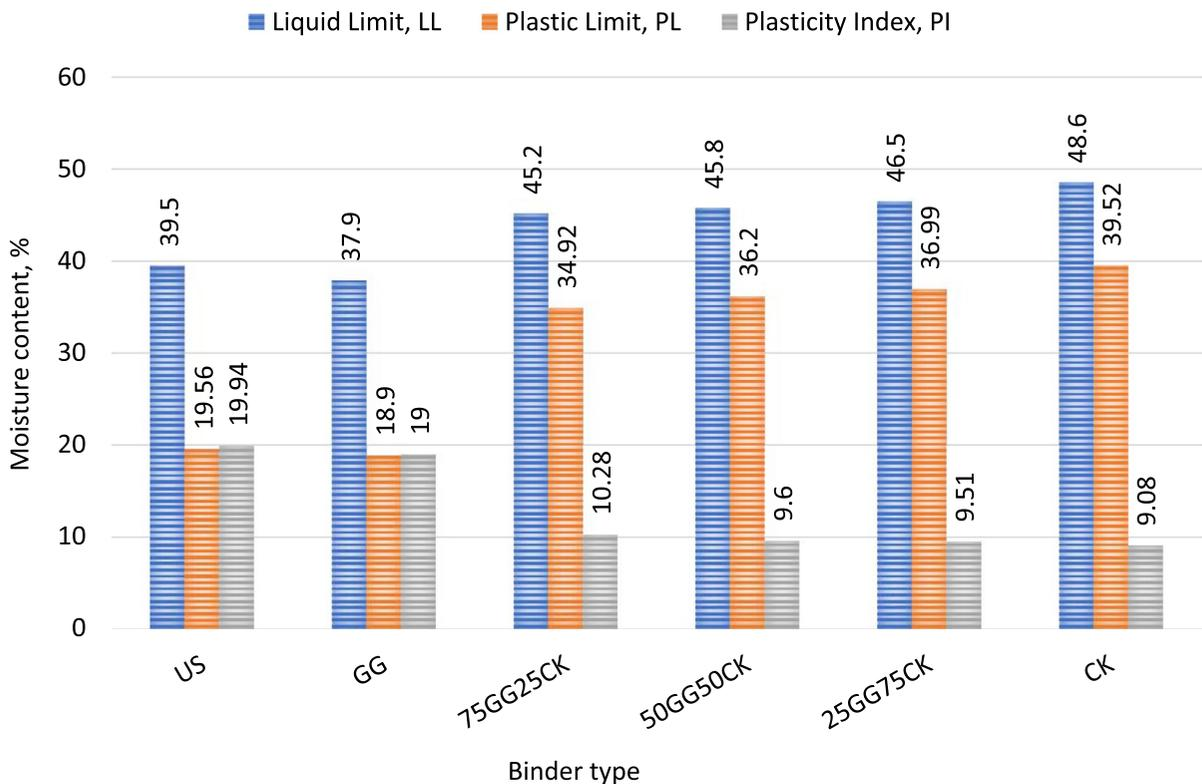
**Fig. 2** Impact of binders on the Atterberg limits of the tested soil
