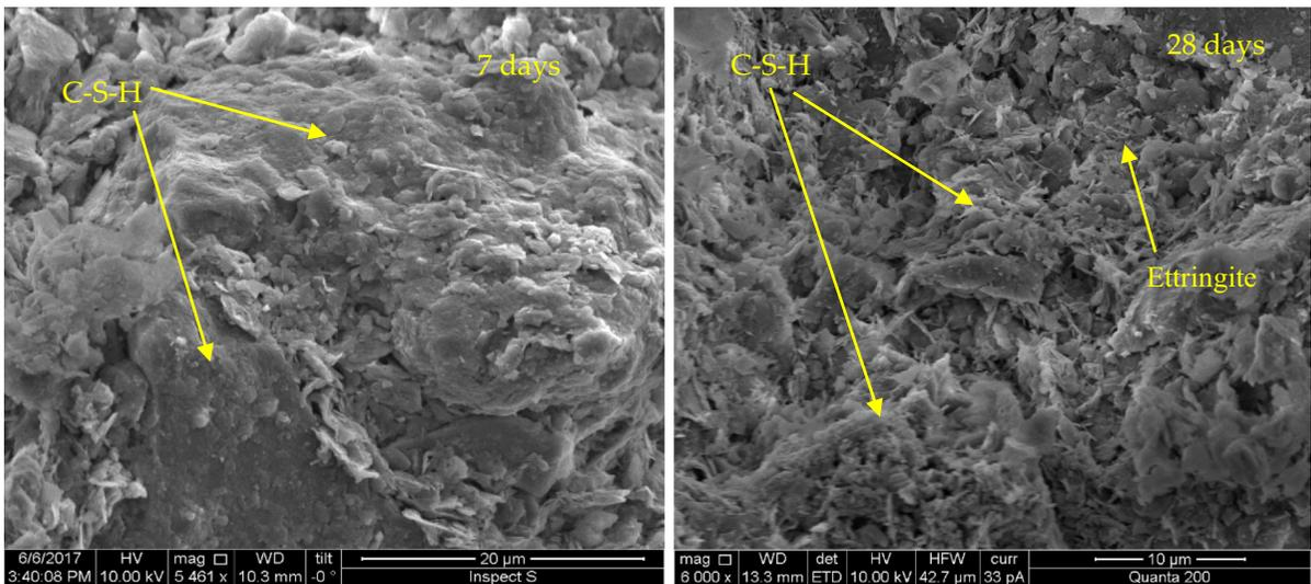
**Fig. 11** SEM image of treated soil with activated optimum binary 25GG75CK binder at **1** 7 days, and **2** 28 days of curing
