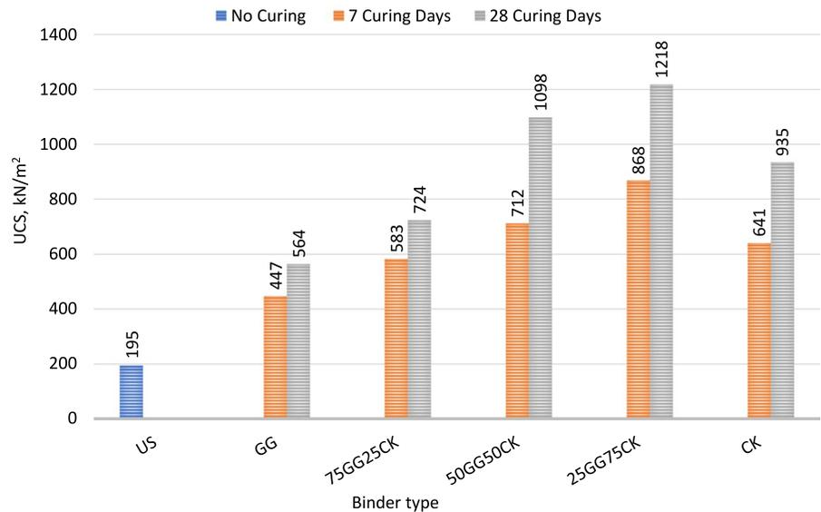
of curing, this binder produced 4.5 and 6.3 times higher UCS than the untreated soil, respectively. The maximal strength gain was similarly found by Konsta-Gdoutos and Shah (2003) when producing mortar from 25% GGBS to 75% CKD. Furthermore, a significant increase in the UCS of soft soil stabilized with GGBS-lime activated binder was documented by Pai and Patel (2018). The strength development was attributed to the formation of the C-S-H product and continuous hydration.
