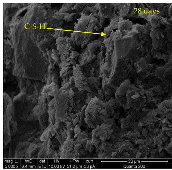
**Fig. 9** SEM image of treated soil with unary GGBS binder at 1 7 days, and 2 28 days of curing
