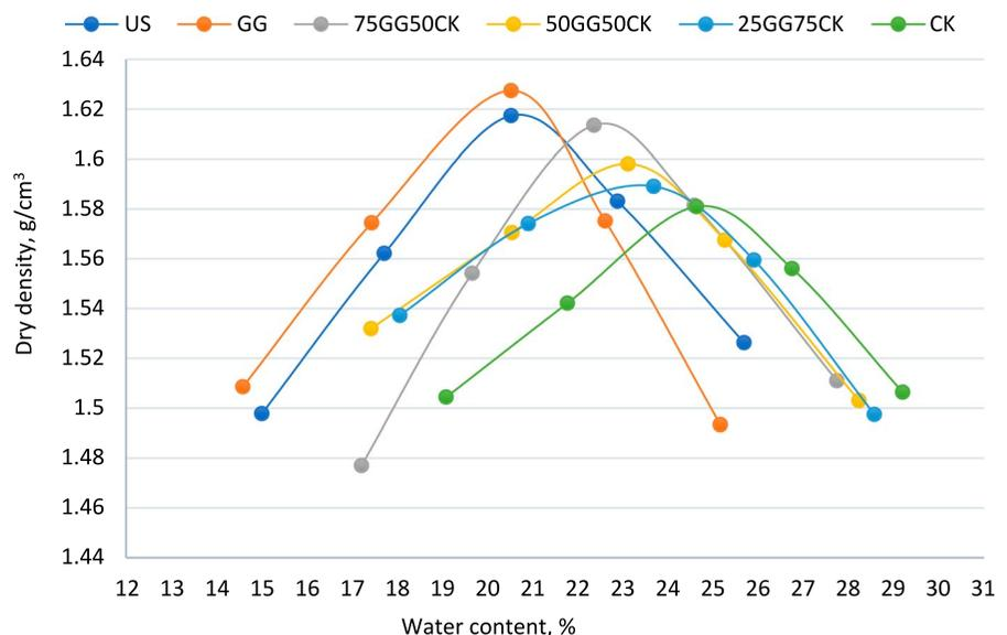
**Fig. 4** Impact of binders on the compaction parameters 1 MDD, and 2 OMC of the tested soil
