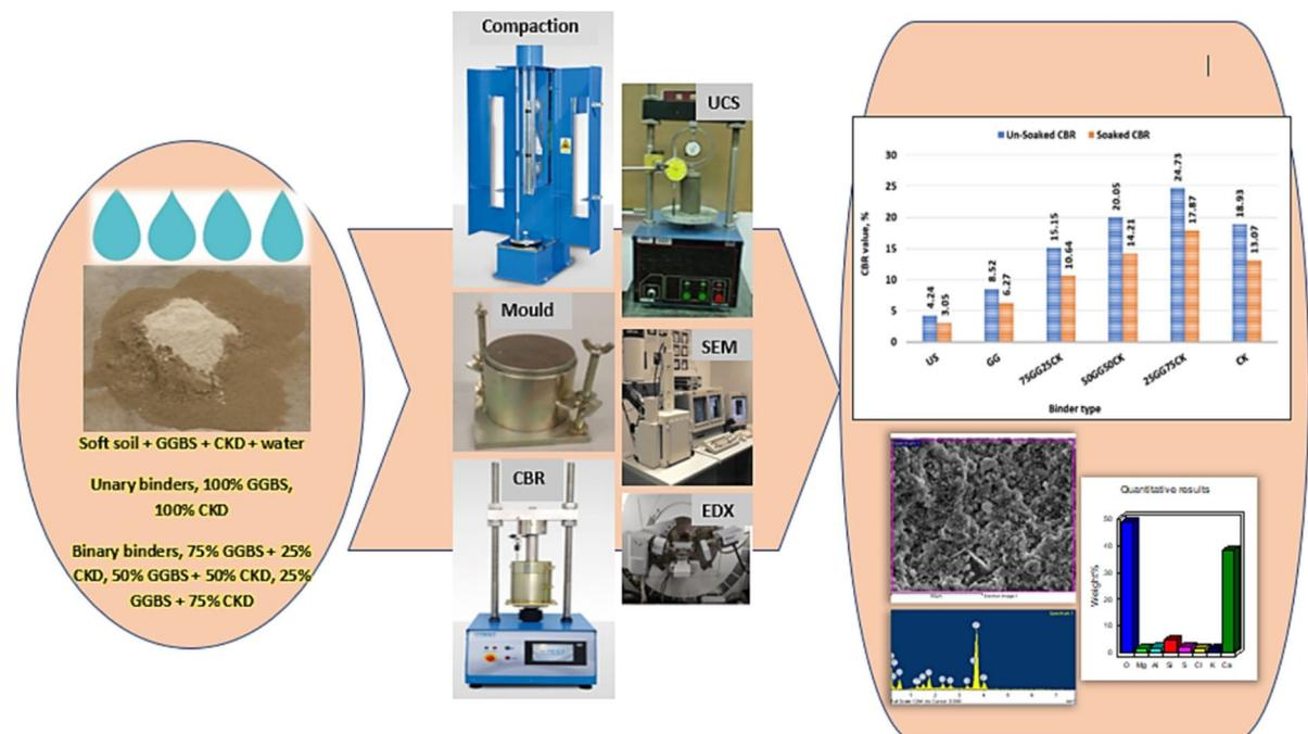
**Keywords** Microstructure · Soft soil · Subgrade stabilization · Sustainability · Unconfined compressive strength
