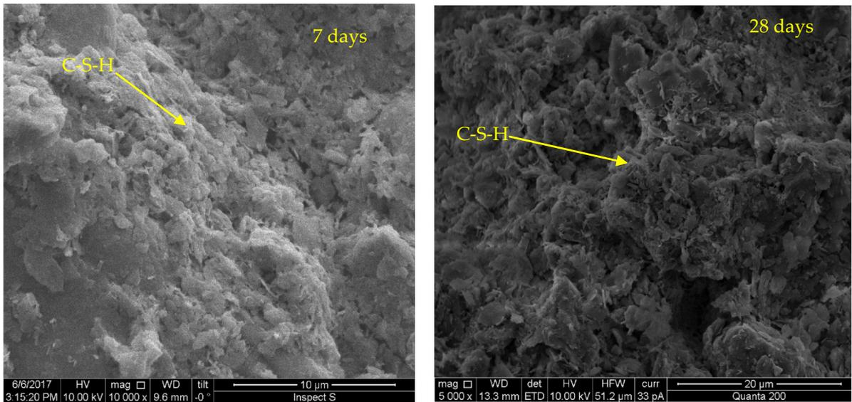
**Fig. 10** SEM image of treated soil with unary CKD binder at **1** 7 days, and **2** 28 days of curing
