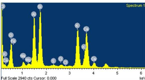
◀**Fig. 7** EDX results of optimum binary 25GG75CK binder paste at 7 days of curing
