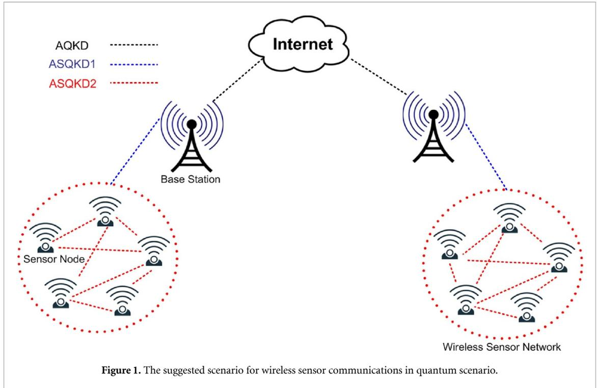
Figure 1. The suggested scenario for wireless sensor communications in quantum scenario.
