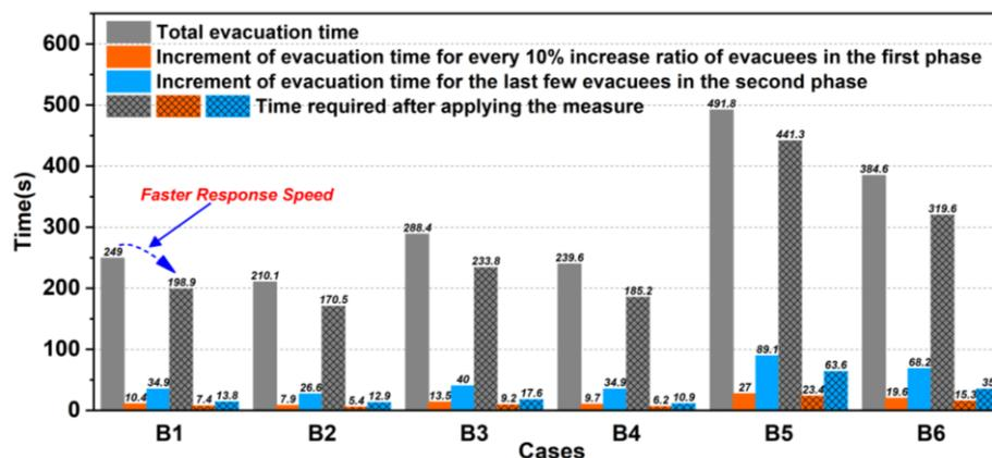
Fig.16 Comparisons after applying the measure “Faster Response Speed”
