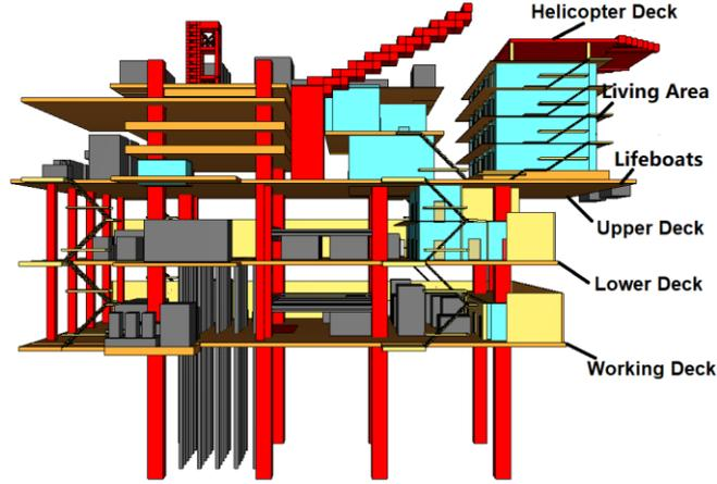
Fig.1 Geometric structure of the selected offshore platform
