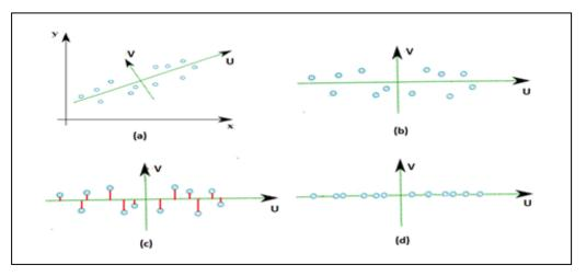
Fig. 1. PCA for two dimensional data reduction: (a) Original data. (b) Data representation. (c) Projection errors using one dimensional PCA. (d) PCA for one dimension dataset
