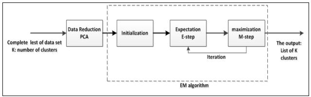
Fig. 2. The model of proposed algorithm
