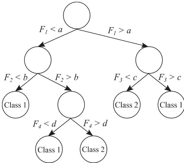
**Figure 2.** An illustration of a binary decision tree classifier. At each node of the decision tree the ‘best’ feature  $F = \{F_1, F_2, \dots, F_n\}$  is used to separate the data by identifying a numerical threshold. After each split-point, the separated data are re-evaluated to select a new ‘best’ feature to further split the data, until the tree reaches a decision at the leaf nodes where the data in each node are assigned a class.
