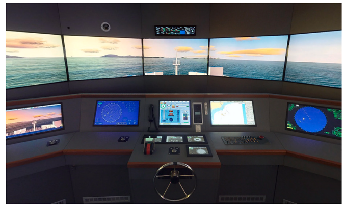
Fig. 3. The ship bridge simulator (Source: the authors).
