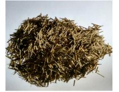
Figure 2. Chopped basalt fiber (CBF) used for reinforcement.
