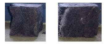
(a) Unreinforced masonry mortar (b) Fiber-reinforced mortar
