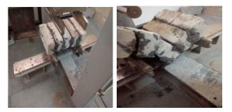
Figure 7. Flexural bond strength of mortar.
