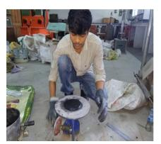
Figure 5. Flow table test.
