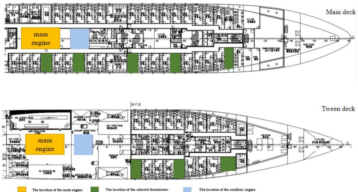
**Fig. 3.** The dormitory layout of the main deck and the tween deck.
