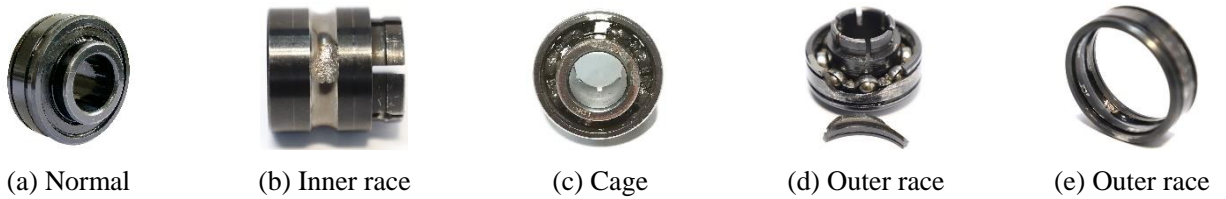
Figure 5: Photographs of the XJTU bearings
