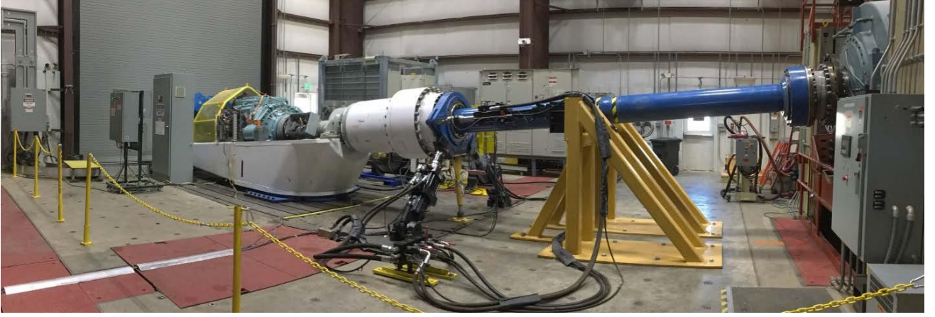
Figure 6: The real wind turbine drivetrain dynamometer installation
