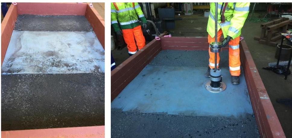
Figure 5. Compaction of sub-ballast (left) and Dynamic Plate Load testing using the LWD
