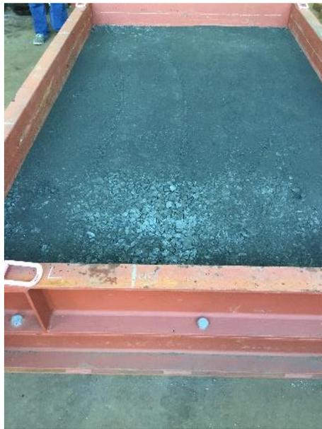
*Figure 6. 400mm height of subballast*
