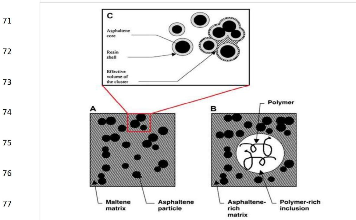
78 Figure 1. Schematic illustration of the colloidal structure of bitumen and the effect of
